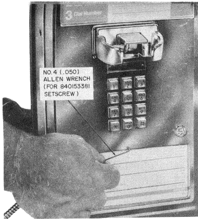
FIG. 1 - Loosening or Securing Instruction Cards (Current Production Sets)
