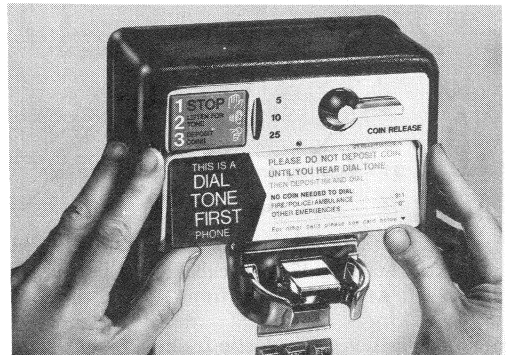
Fig. 20—Installing Instruction Cards in 1-Type Set (Typical)
