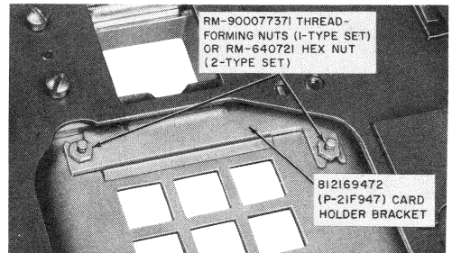
Fig. 29—Card Holder Bracket Installed in TOUCH-TONE Set
