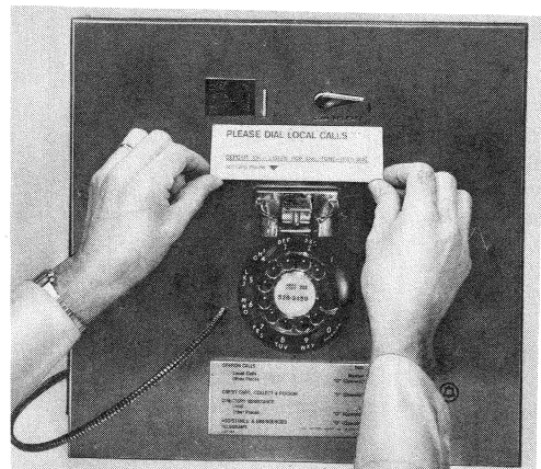
Fig. 25—Installing Instruction Card in 2-Type Set With Cam
