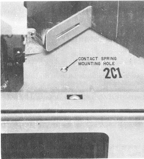
Fig. 9—Location of Contact Spring Mounting Hole in 2A, 2C, or 2D Telephone Sets
